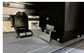
Printhead Anti-Collision Protection
