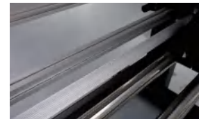
Tension Dancer Roller ensures smoother and flatter film feeding
