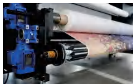
Y-direction stepping motor for higher precision
